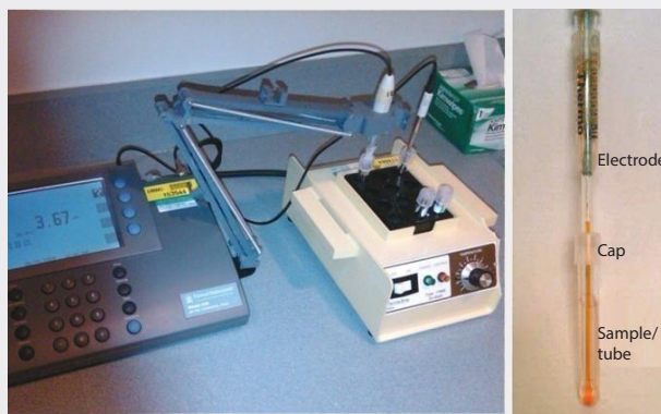
FIGURE 3D.1 Example setup of a pH meter and electrode for measurement of culture media pH. A warming block is used to account for the impact of temperature and is set to ~37°C. The electrode is placed through the cap to prevent excessive gas exchange that could affect readings. The electrode/cap is removed from the storage solution tube, calibrated, and then quickly placed into the tube of medium for measurement.
